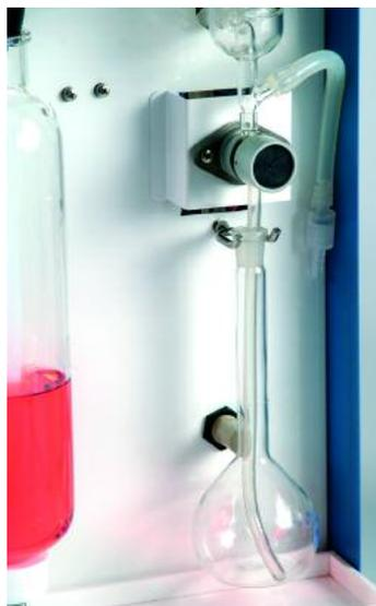
*Automatic termination of final distillation at 200 ml of distillate. By using the ADD function small quantities of distillate can be added to accurately fill the matrix flask to the mark without having to add water to the distillation.*
